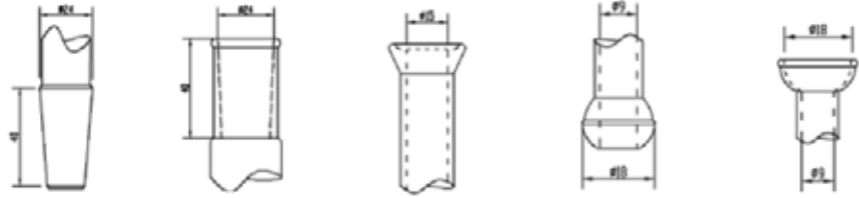
Standard Dimensions for Full Length Interchangeable Taper-Ground Joints
